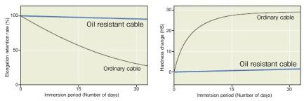
%Oil resistance is based on test results, not a guaranteed value.
