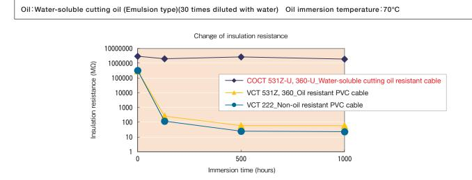
\*\*Allow it to cool naturally until the test oil drops to 25°C after immersing the cable for the specified time. After the oil temperature drops, the insulation resistance is measured with the cable immersed in the test oil. Test results are not guaranteed values.
